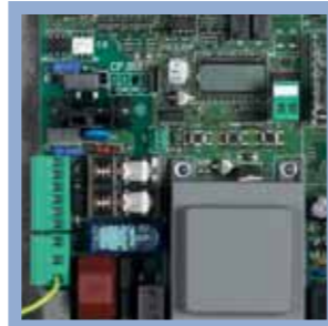
Control unit with advanced programming on display. Built-in receiver and removable terminal boards
